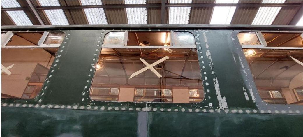
Large saloon glazing. Note the countersink holes, all of which needed to be filled and sanded
