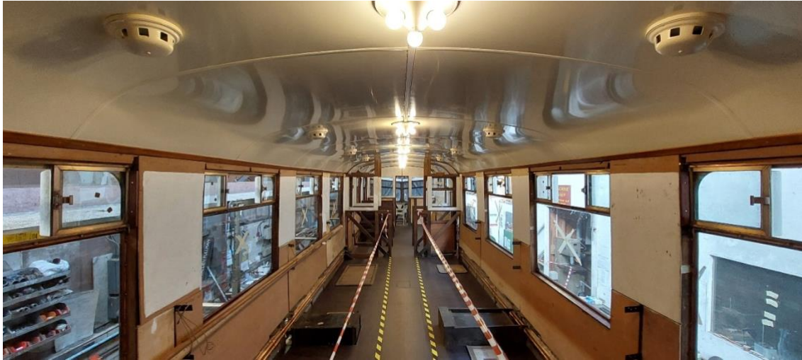
Main section of ceiling panels installed with the original vents and lighting clusters fitted
