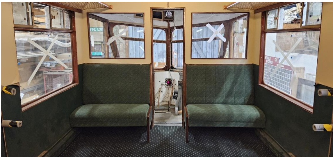
Seating installation progressing in the small saloon with the green carpet in place (Also visible are the fitted restored luggage racks)
