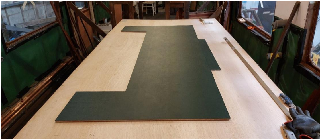
Leathercloth applied to side panel ready for fitting
