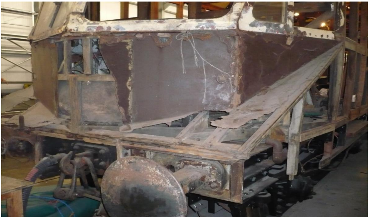
Badly corroded state of the cab metalwork before reconstruction
