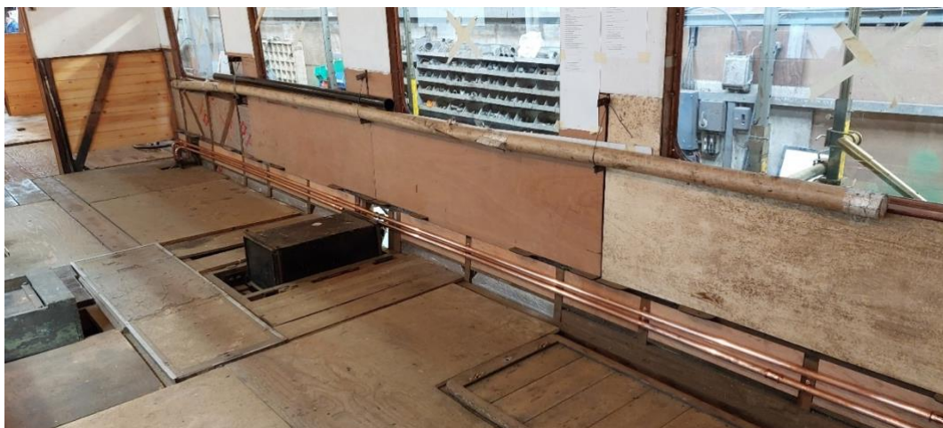
New pipework installed within the large saloon, replicating the old heat pipe layout
