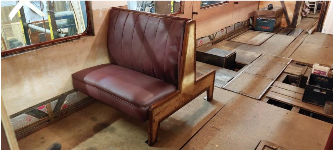
The existing seats, with the incorrect leatherette covering and non-compliant horsehair filling
