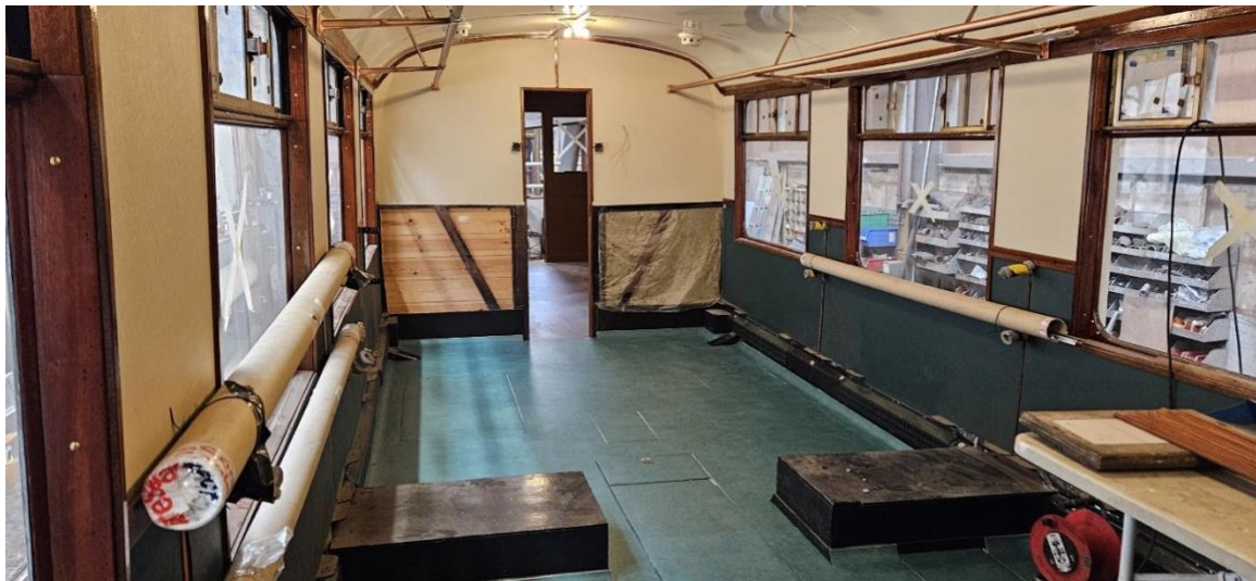
Green Marmoleum laid in the large saloon, just awaiting the seating
