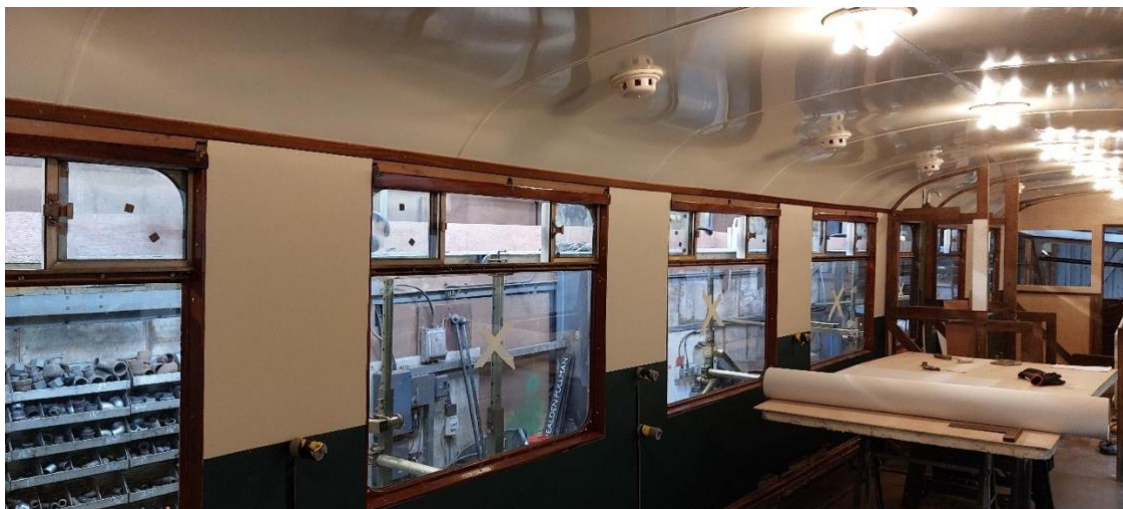
The cream upper and green lower leathercloth panels fitted within the large saloon
