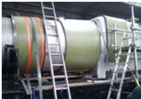
Cladding being fitted to 4253's boiler. (via 4253)
