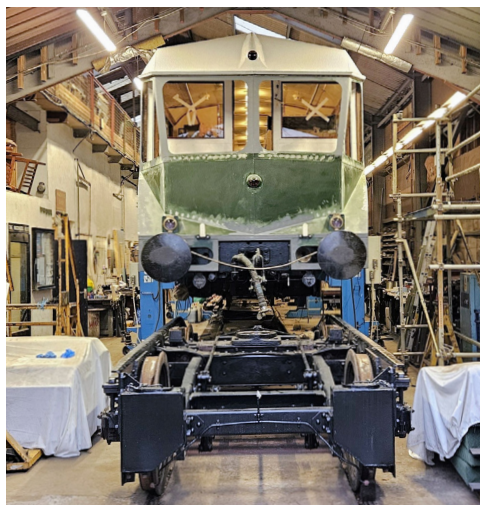
The bogie going back under the Railcar. (Neil Edwards)
