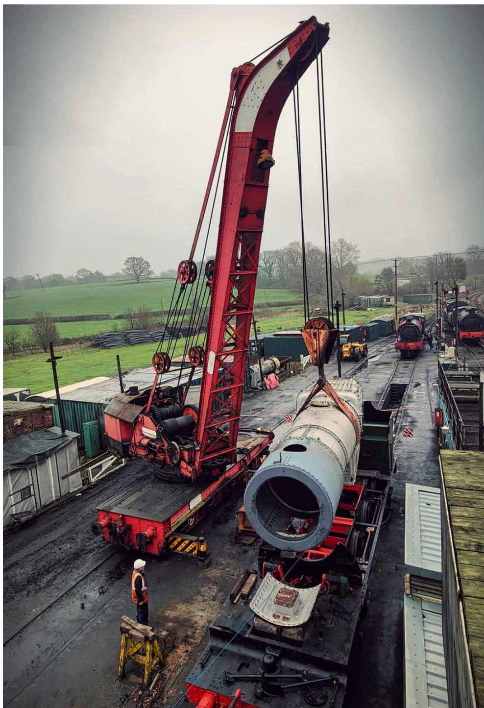
The big lift – 4253 gets its boiler.
