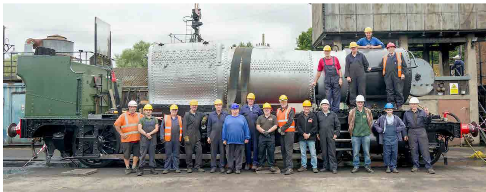
Members of the 4253 team celebrating as the loco's boiler is temporarily fitted to the frames for the first time. (via 4253 Locomotive Company)
