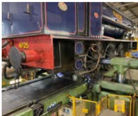
No.25 having its wheels turned on GWR's lathe. (Martyn Pearce)
