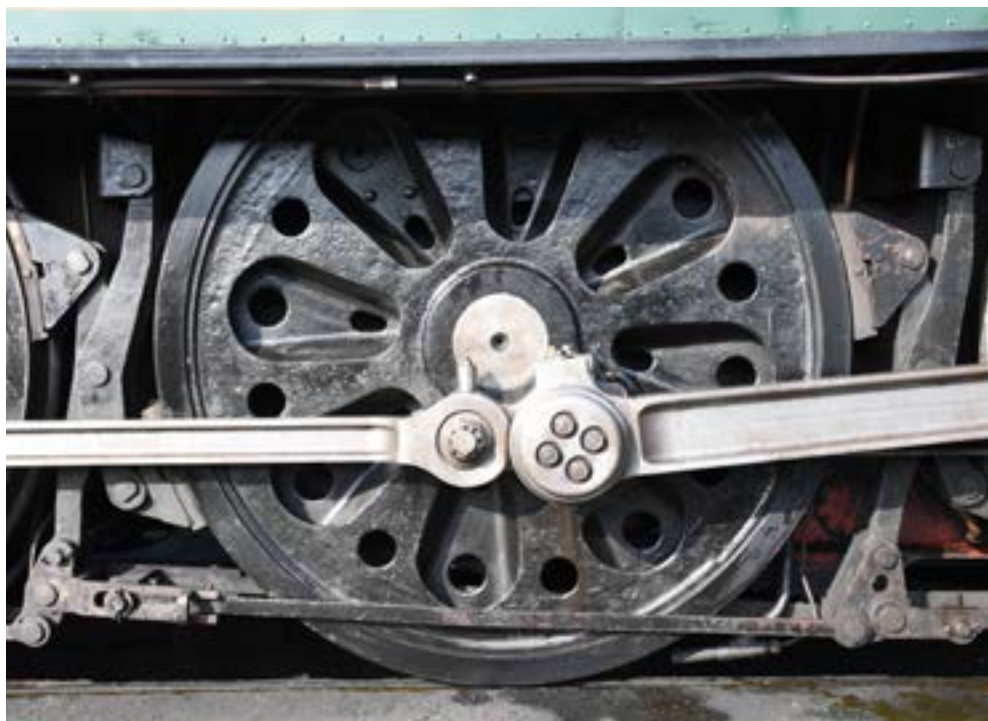
Bulleid Firth Brown middle driving wheel on 257 Squadron.
