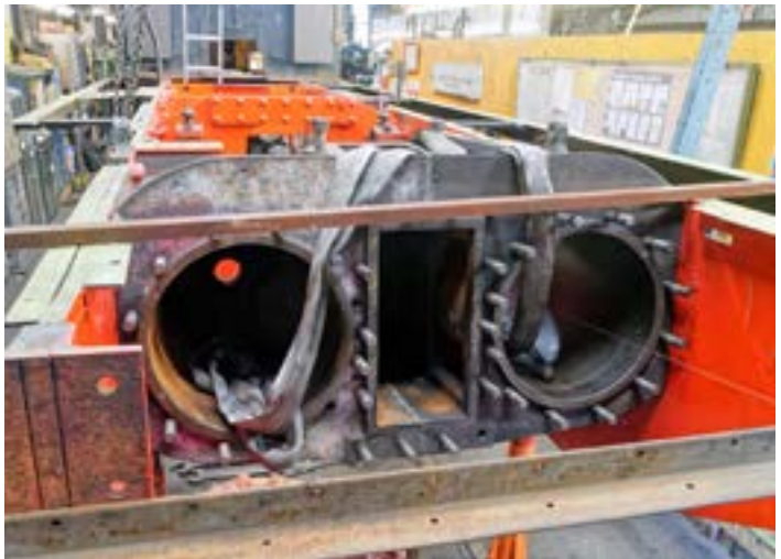
Charwelton's new cylinder block in place.
