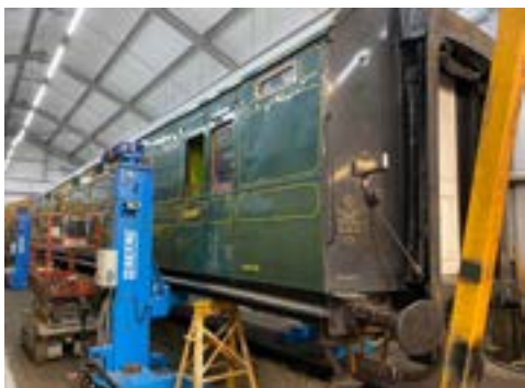
NBO 53 up on jacks for the bogies to be removed. (Mark Stuchbury)
