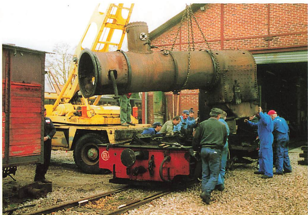
Return Ticket to France: K&ESR volunteers remove boiler from CFBS Locomotive No 25 at St Valery, 20th November 2004 (upper) and CFBS volunteers pay a return visit to the K&ESR C&W shed on 6th February 2005 (John Liddell)
