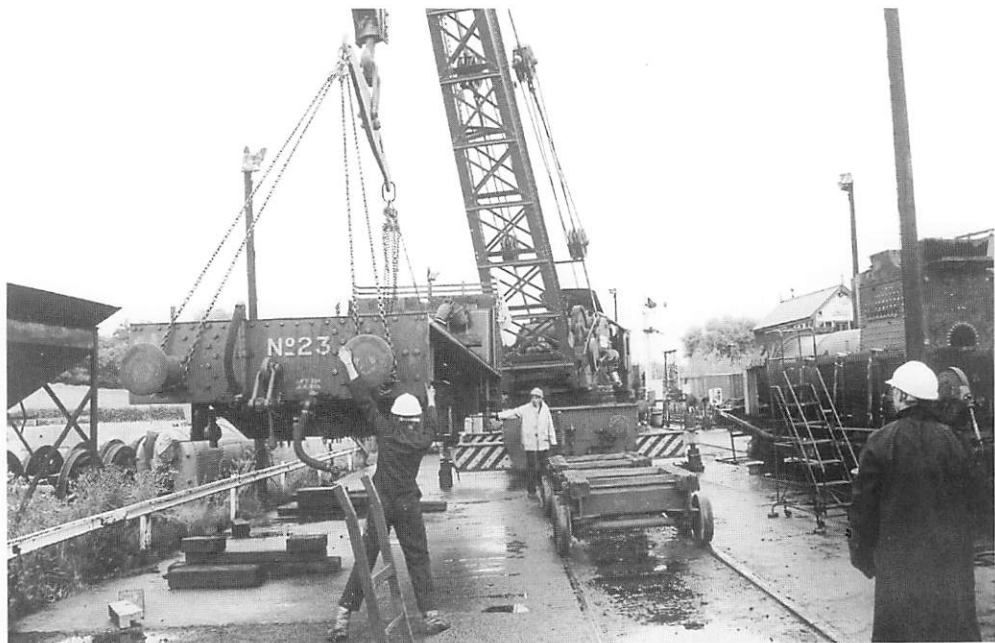
36ton crane lifts the frames for No 23 on to the prepared accommodation bogies, 6th August 2000 (John Liddell)
