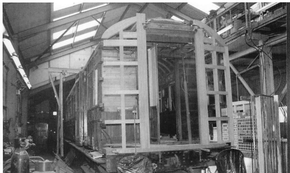
Maunsell BNO No 4432, showing the extent of restoration necessary on the Headcorn end vestibule, 6th June 1999.
