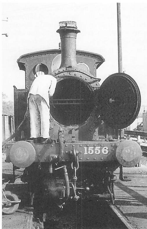
The Last Day. 1556 passes Orpins Curve, returning to Rolvenden prior to withdrawal from service, and below, the smokebox is cleared of ash for the last time. (Neil Rose)
