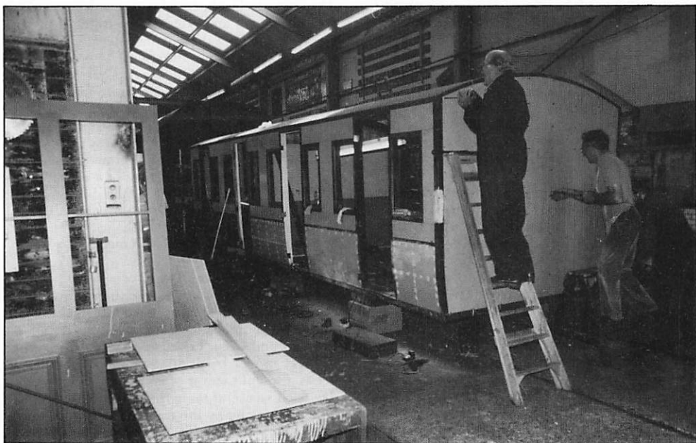
The SE&CR 4-wheel coach (from Ashford) undergoing re-building at Tenterden on 5th August 1994.
