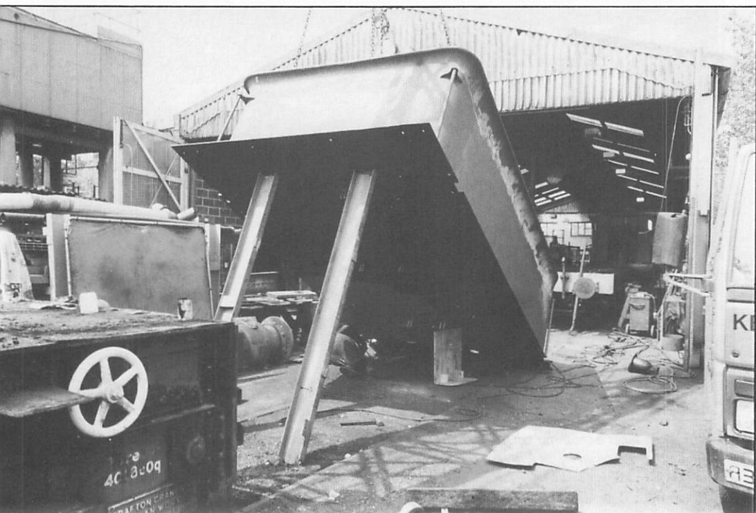
No. 19 "Norwegian" undergoing restoration at Rolvenden on 22nd July 1994. The tender is being suitably supported so that the underside can be painted. (John Liddell)
