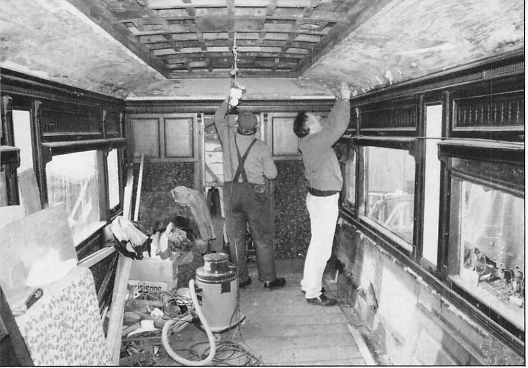
Frank Kent and Ken Lee stripping the main saloon ceiling ready to take the new wallpaper. Note at the end are the two remaining panels covered in the previous dark green moquette. Through the end door is the luggage compartment. 31st January 1993. (John Liddell)
