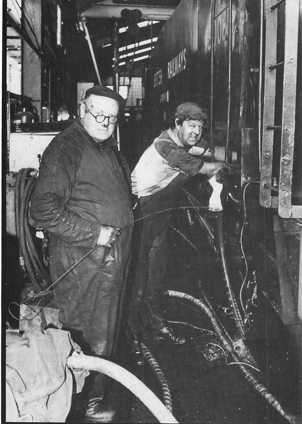
Locomotive Department Manager, Bob Forsythe (left) and Bernard Sealy carry out a boiler washout on No. 22 "Maunsell", 25th August 1990.
