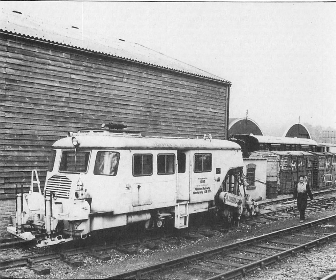
The recently acquired Plasser & Theurer tamping machine, 25th August 1990.
