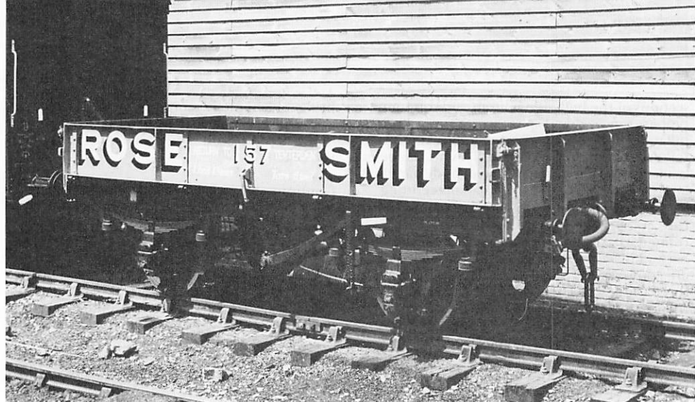
Newly restored steel-sided dropside wagon bearing the name "Rose Smith", after a Company that once traded by rail to Tenterden (Brian Stephenson)
