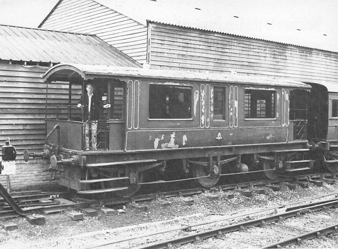
Ex L.N.W.R. saloon 40 years later at Tenterden, 18th August 1985. Gas lights now removed, modified running boards and fixed lavatory window [Brian Stephenson]
