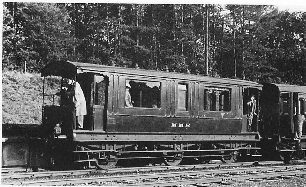
The ex L.N.W.R. Saloon at Longmoor, 10th August 1946 still in Melbourne Military Railway livery. Note gas light roof vents, continuous running board and hinged lavatory window [H.C. Casserley]
