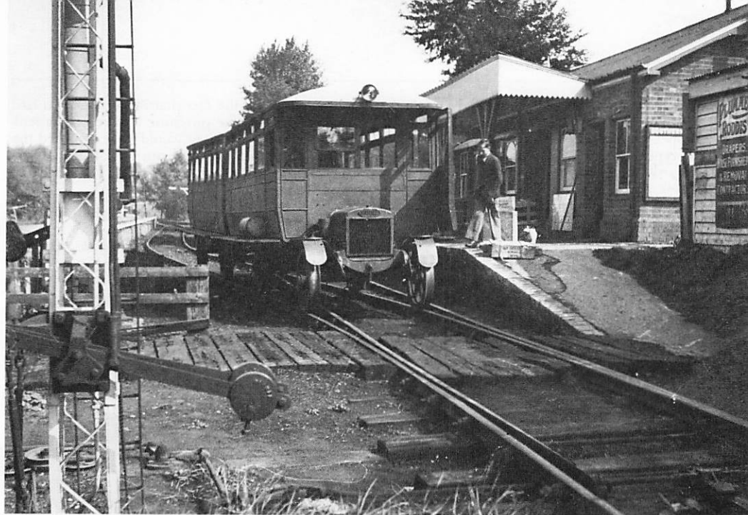
At Tenterden Town resting on the loop points. Note headlamp now moved from conventional position to the roof and buffing gear removed. [Eric Graves Collection]
