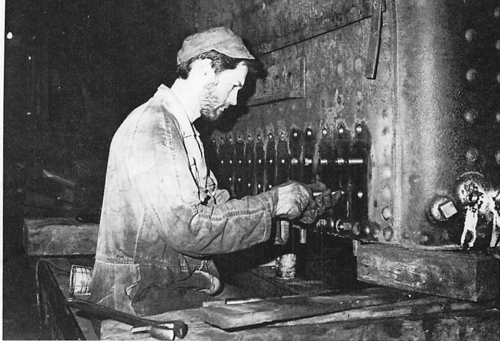
Lawrence Donaldson replacing firebox stays in "Linda's" boiler, 4th May 1985
