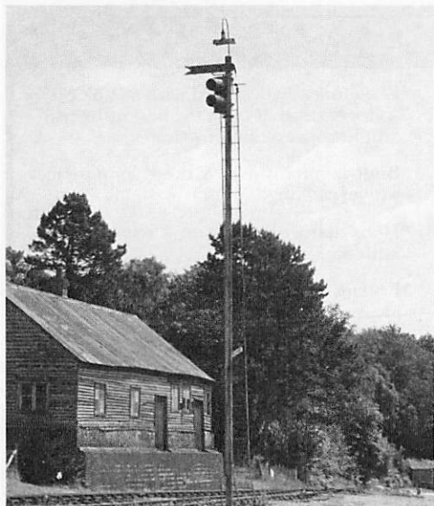
The disused semaphore and two aspect colour light signal which superseded it protecting the exchange sidings.
