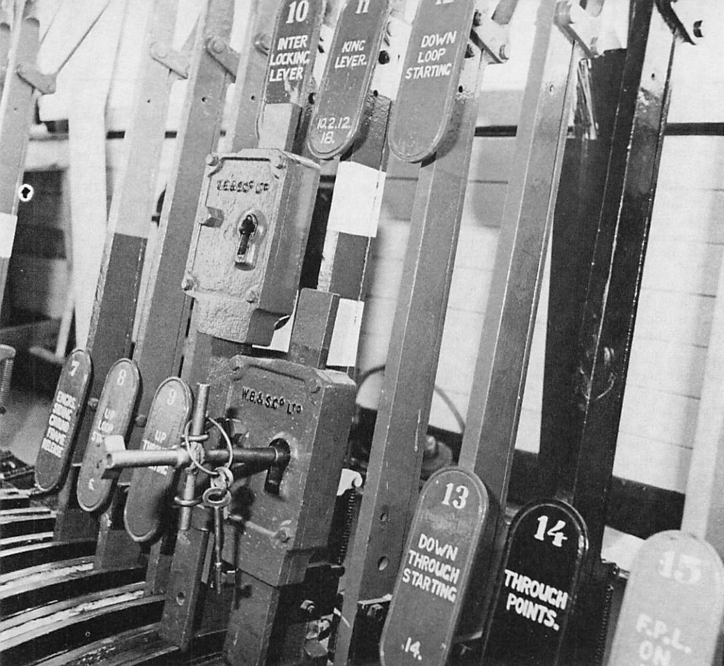
Wittersham Road signal box with the frame opened and the long section staff shown locked in. The medium section staff is placed in lever 10 for the box to be closed [Jim Berryman]
