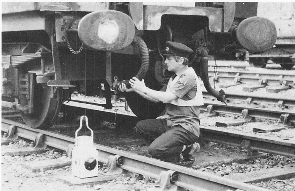
The Author carrying out a brake test.
