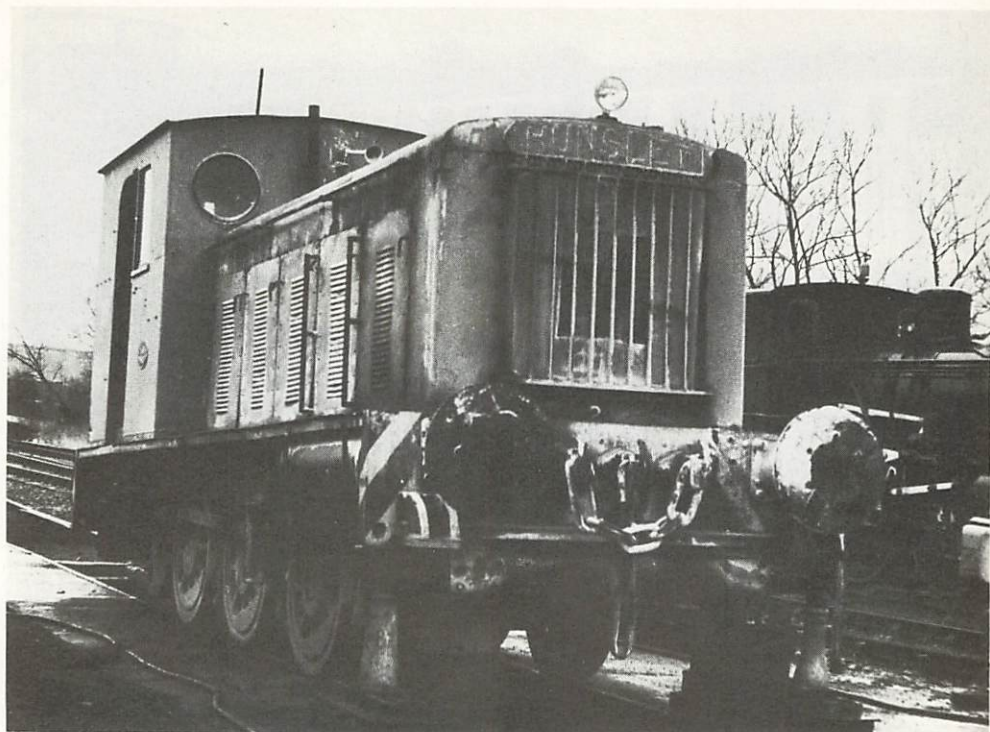
Hunslet 0-6-0 diesel locomotive , jacked up for axle box inspection at Rolvenden, February 1978. [Donald H. Wilson]
