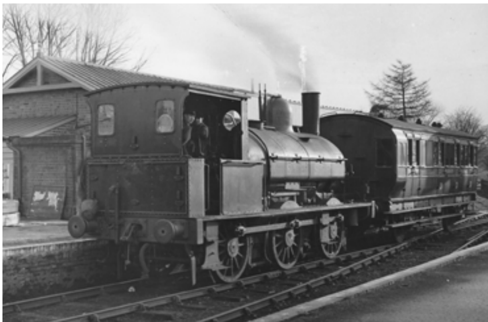
No.4 at Tenterden on 27th March 1937, probably on a railmotor replacement service. This ex-LSWR (SR) 'Saddleback' was exchanged for 0-8-0T Hecate in 1932 and took that locomotive's number, but not its name. Later in 1937/38 she received a different boiler and ran until nationalisation. (Ron Jarvis/CSRM)
