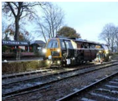
Tamper to Tenterden. Waiting to align the relaid platform road. (Alan Crotty)
