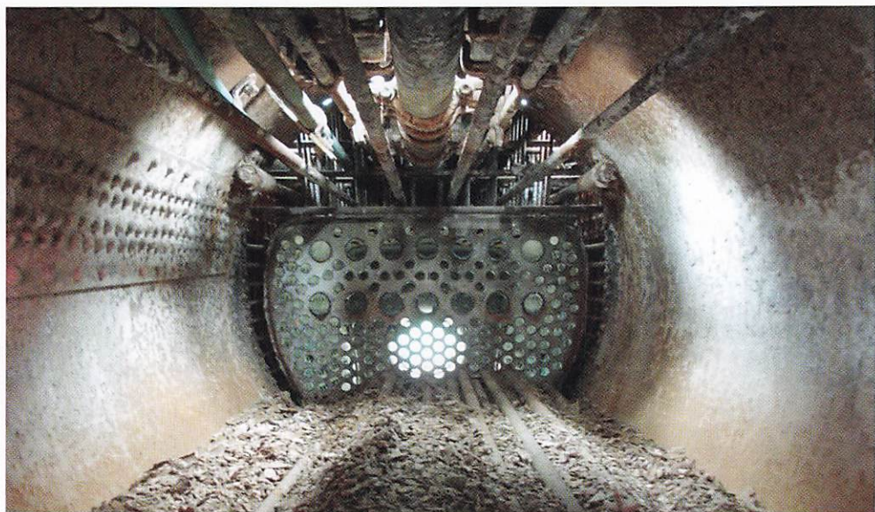
Most of the tubes removed, and a vast amount of scale still inside the boiler. (4253 Locomotive Co. Ltd.)
