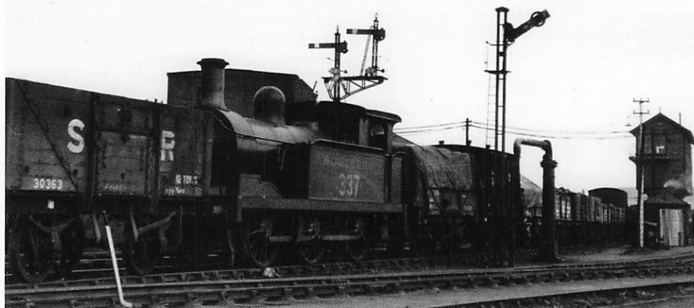
Southern Railway R1 0-6-0T No.A337 shunting at Maidstone West in 1932. The signal in the foreground controlled access to the Tovil branch. (Andy Hardy collection)
