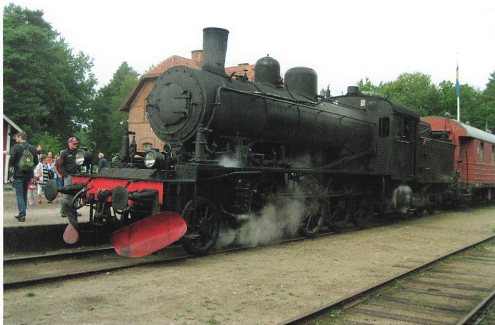
Originally a 0-8-0 of 1914, this loco was rebuilt as a 2-8-0 in 1948.
