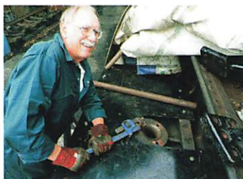
Dick Beckett removing broken cylinder studs from 4253. (Charlie Masterson)
