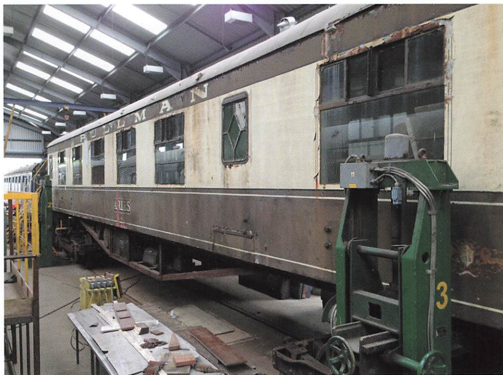
Aries on jacks at Rampart Engineering with underframe works in progress June 5, 2013 (Andre Freeman)
