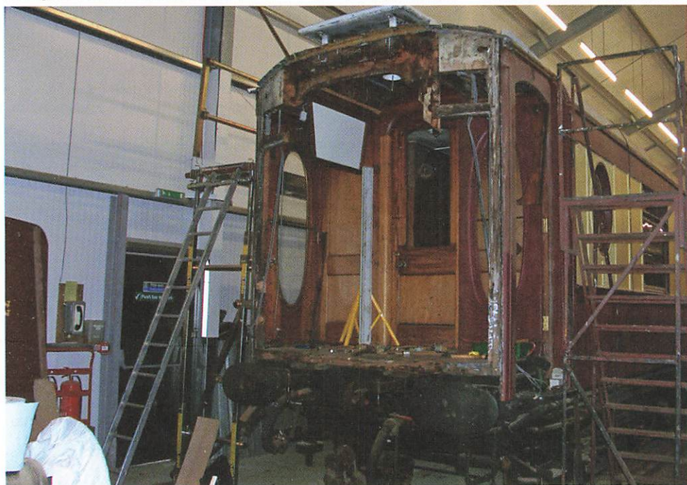
Don't Panic! 'Robertsbridge' end of Barbara being prepared for replacement timbers. The paintwork is undercoat - not a sign of a 'Blood and Custard' Pullman (Nick Pallant)
