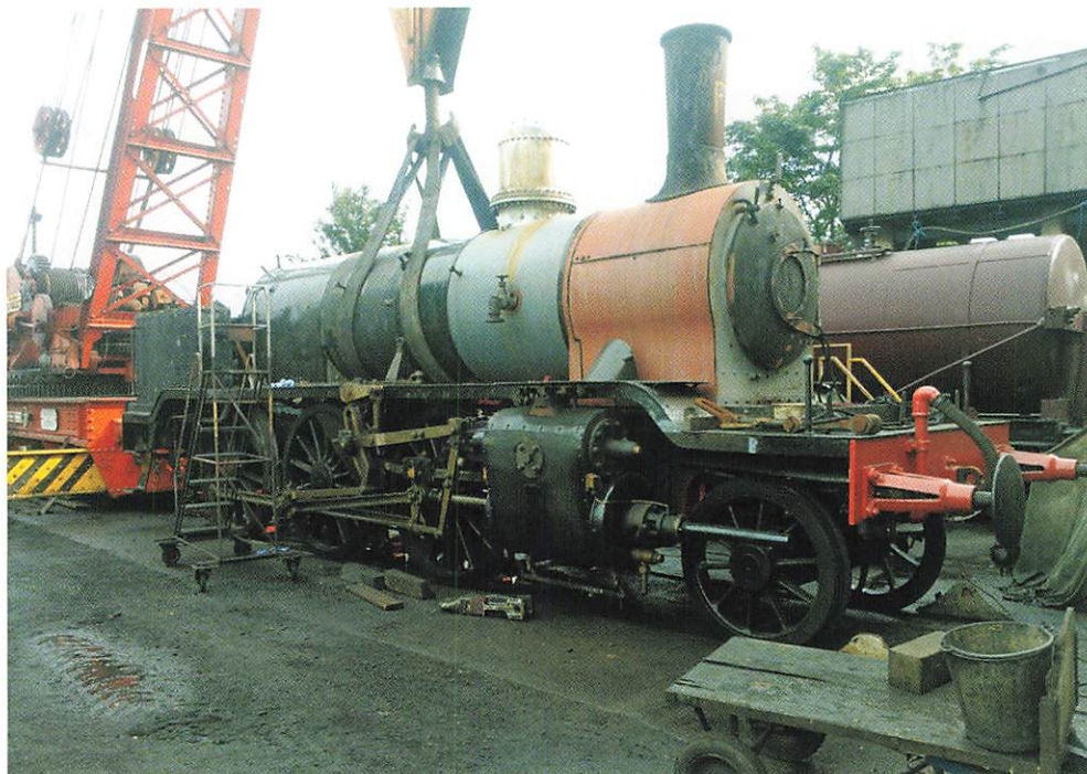
Norwegian's boiler being lifted into the frames (Paul Wilson)
