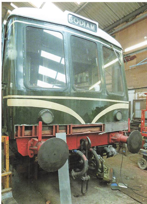
DMMU Bodiam end car under repair in Carriage & Wagon(Duncan Buchanan)
