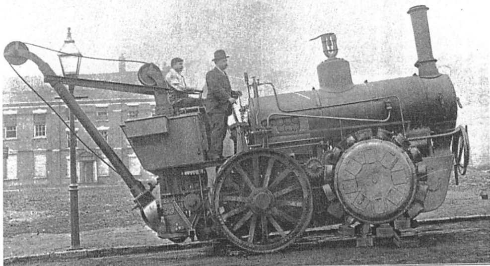
The four-wheel-drive Kerr-Stuart engine with lifting gear under trial in January 1902 (Pedrails on front axle only)
