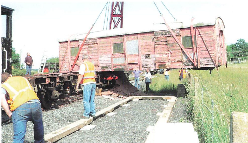
Lifting the PMV body at Bodiam. (John Liddell)
