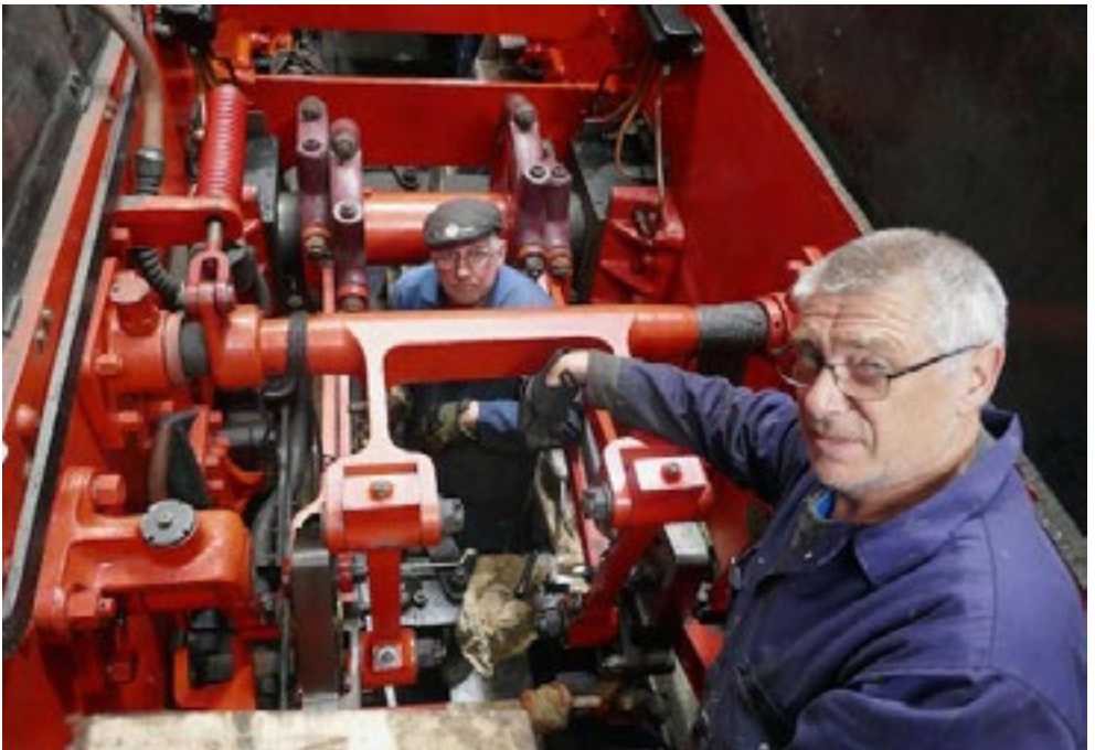
Dick Dickson (left) and Kelvin Williams assembling the last of 4253's inside motion. (Charles Masterson)
