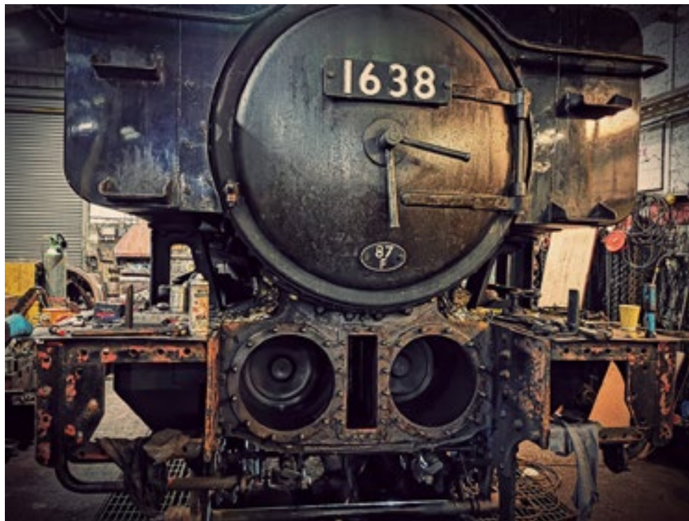
1638 receiving attention to its pistons and valves.
