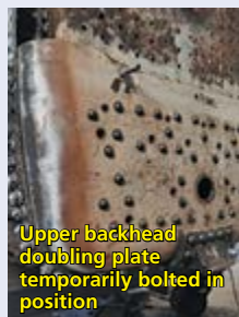
Inside of firebox, showing stay holes
